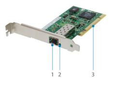
1. Fiber Ports 2. LED Indicator (Link / Activity) 3. PCI Slot
